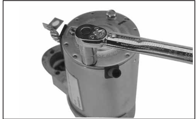
Figure 8-55. Serrage des boulons.
