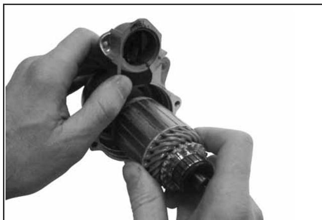
Figure 8-21. Installation de l'armature.
