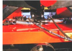
HYDRAULIC REMOTE CONTROL Accurate shutter open and close from tractor cab.
