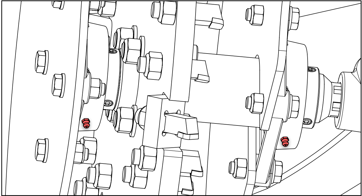
Flywheel Shaft Bearings (Underside of Flywheel Housing)
