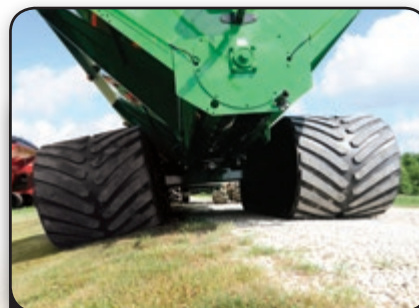
Equalizer® tracks are independently cambered to follow ground contours for optimum flotation
