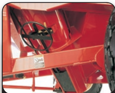
Lockable wheel-operated cleanout door for easy cleaning between crop types
