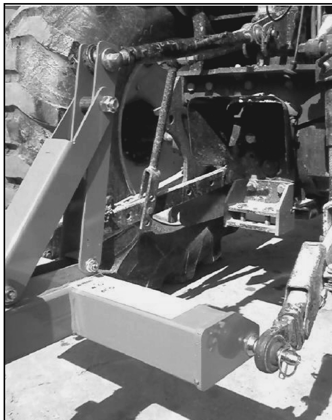
Figure 1. Lower Lift Arm Attachment and Top Link Connection, Category 1
