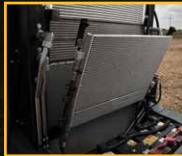
Just pivot the front plane of the cooling package out of the way to remove debris from the second plane containing the radiator.
