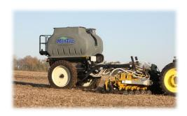
GEN II Base Unit with gray bins on a Montag Auto-Steer Cart shown above. Other color options include white and yellow. Bins have two fill inlets each and are independently scaled. All units use the Montag particulate metering system. Multiple U.S. and international patents cover either, or both, this Product and its components.
