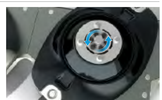
Overload element shears off – mower disc turns freely – drive is protected
