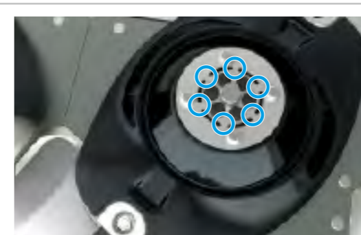
Mower disc is jammed
