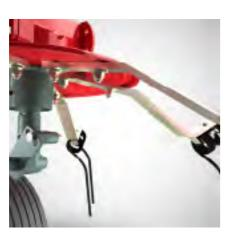
The tine arms are made of tough, galvanised flat steel bar, which allows a wide contact surface between tine and rotor plate. This ensures very good power transmission even under the harshest of working conditions. The forces are optimally absorbed whenever the ground is uneven.
