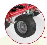
**ACCURATE DETECTION OF THE GROUND CONTOURS** The contact wheel with balloon tyre ensures optimum ground adaptation (special equipment).
