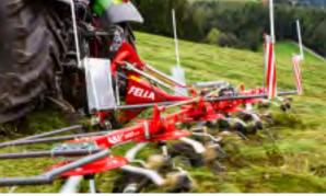
OPTIMUM GROUND CONTOUR FOLLOWING **ON SLOPING TERRAIN** The patented, low-lying towing point guarantees excellent trailing behaviour and prevents downhill travelling.
