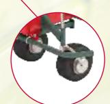
ADJUSTED TO SUIT THE GROUND The movable contact wheels (available as an option) optimise ground sensing and ensure tidy raking and protection of the sward.
