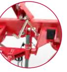
**ALWAYS AT THE RIGHT HEIGHT** The working height can be adjusted centrally using a spindle.
