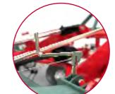
ALWAYS AT THE RIGHT HEIGHT The working height can be adjusted centrally using a crank.
