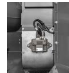
Fewer and shorter stops for unloading are soon reflected in a greater daily yield – sensors for yield and moisture and a grain quality camera are fitted to the elevator. The data is accurate to 98%, and applied with the VarioDoc ISOBUS standard, live yield mapping and IDEALharvest™.
