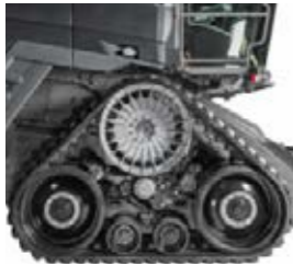
The TrakRide crawler drive minimises ground pressure.
