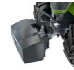
Using the comfort ballast pickup, front weights can be picked up quickly and easily, even without front linkage.
