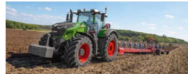
Thanks to the TMS tractor management system and the automatic maximum load control 2.0, the tractor adapts the engine speed optimally to the road speed.
