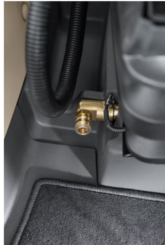
The cab is cleaned quickly: The driver seats (super comfort seat Evolution) have a practical connection for a compressed air hose, which can be used to clean the cab.
