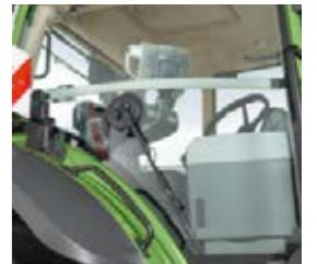
The 220° side window wiper also guarantees an optimal view to the right side, even in adverse conditions.
