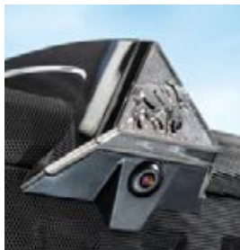
Practical for front mounted implements: The new camera integrated in the bonnet captures the view to the lower links and transmits the image to the Varioterminal.
