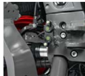
The Fendt 1000 Vario provides connections for up to seven control units, six at the rear and one in the front.
