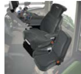
The super comfort seat Evolution dynamic has air-suspension and active climate control as well as a backrest extension.
