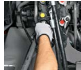
The self-closing valve flaps protect against contamination and enable one-handed coupling.
