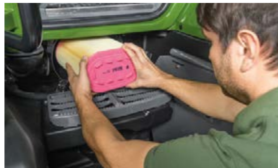
The cab filter is easily accessible in the entrance area and can be easily cleaned when needed.
