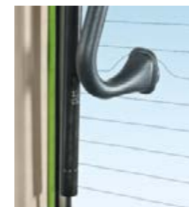
The front and rear windows are heated, which is a big advantage when operating with the reversing driver station.
