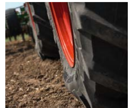
The perfect integral tyre pressure regulation system VarioGrip controls tyre pressures from 0.6 to 2.5 bar within minutes. The optimal tyre pressure saves fuel, protects the soil and increases traction.
