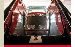
The main loader arms are constructed of two U-shaped, high-strength alloy steel channels fitted together and welded on the inside for a wide profile with a clean, strong appearance.
