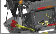
Dual SCH (Schumacher) epicyclical drives provide smooth positive power, Increased cutterbar performance and greater power efficiency over belt or hydraulic drives.
