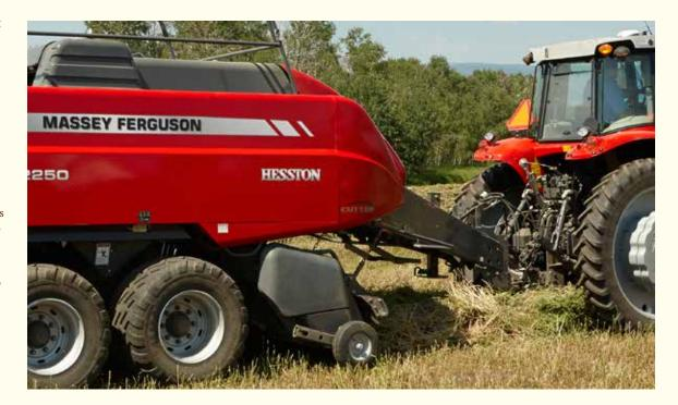
To help produce rock solid, well-formed bales and uniform density, we've also extended the length of the OptiForm™ bale chamber on the Hesston 2270 XD and the 2290 — by a full 16 inches.
