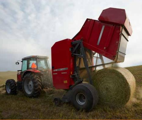
With a wide, low-profile pickup and centering augers, the Hesston 2900 Series tackles wide windrows with ease, while maximizing leaf retention. And by packing the chamber all the way to the edges, the result is dense, square-shouldered bales.
