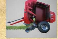
**Open-throat feeding** assures high-capacity baling on all Hesston round baler models. As the pick up gently moves the hay into the chamber, the forming belts and starter roll begin rolling the all-important bale core.
