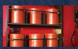
**The large twine box** adjusts to hold eight 20,000-foot balls or twelve 10,000-foot balls, so you can keep baling all day long. The convenient location allows easier access to the baler drives.
