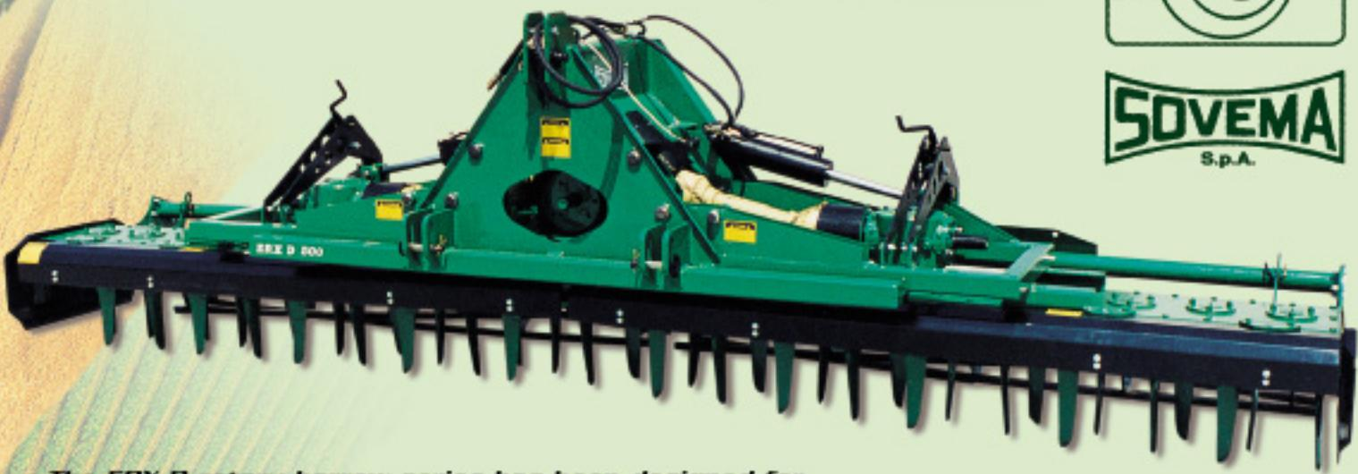
The ERX-D rotary harrow series has been designed for large Farmers and Contractors. On a very strong frame are mounted two special rotary harrows, powered by PTO shafts, directly connected to the main central gearbox. For road transport, the two rotary harrows are hydraulically lifted, directly from the tractor driver's side.
