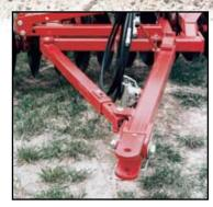
The precisely positioned hitch is adjustable to help you fine tune your disc so it will pull straight in nearly any field condition. This, combined with a pre-set gang angle makes the 1300 the straightest pulling offset on the market today.
