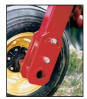
Wheel adjustment on the center section of the 1331 or main frame of the 1321 is an essential adjustment. It allows the frame to be leveled to meet existing field conditions.
