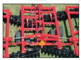
1435-21' through 29' features a wider center wheel placement for improved road stability and field performance.
