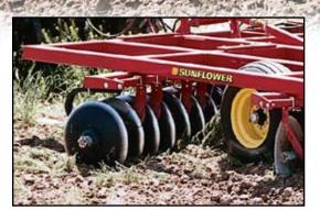
Available with 22", 24" or 26" disc blades in 8 1/2" spacing, which enhance residue coverage and increase ability to penetrate the soil. Large 1 3/4" gang shafts with a spring washer on the ends of the gangs, provide a solid foundation for maximum gang performance.
