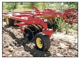
Heavy-duty swivel type gauge wheel turns with the disc instead of creating a furrow or bending due to side loading found on rigid mounted gauge wheels.
