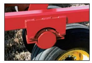
The lift systems are equipped with replaceable ductile cast iron bearings. The top casting features an X-groove that allows grease to flow over the entire bearing surface for increased life.
