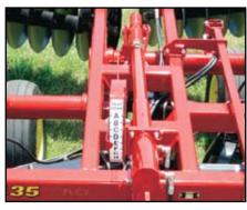
An optional hydraulic front-to-rear leveler allows the operator to fine tune the 1435 from his tractor's seat. A well-adjusted disc not only pulls easier, but leaves the field in better condition.
