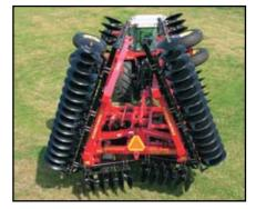
Available with 22" or 24" disc blades with 8 3/4" spacing, which enhance residue coverage and increase ability to penetrate the soil. Large 1 3/4" gang shafts feature a gang nut on each end as well as spring end washers to provide maximum gang performance.
