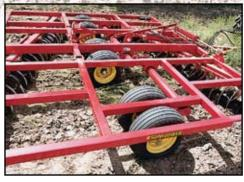
In-line wheel placement provides a stable platform for uniform penetration and precise leveling.
