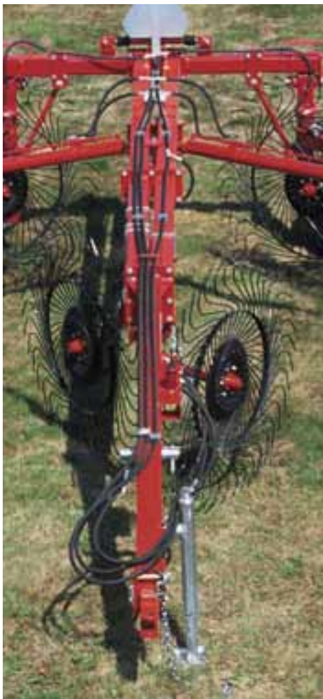
▲ Open up the center of a windrow with center kicker wheels to speed drying.
