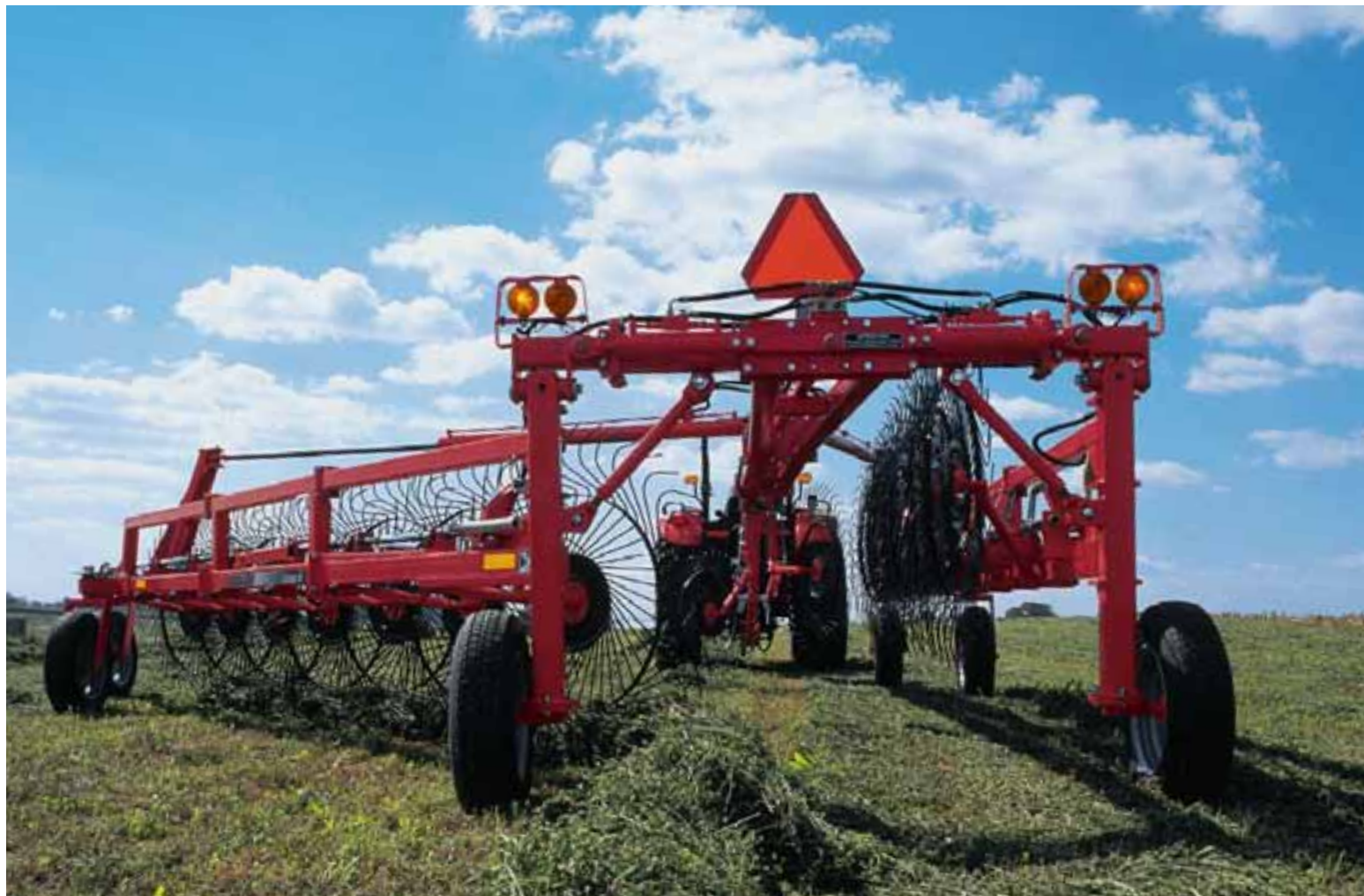
▲ Optional single side opening kit turns damp windrows for faster drying
