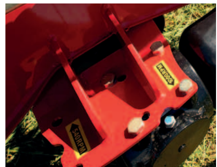
These machines can be operated with either 540 or 1000 rpm without additional accessory.
