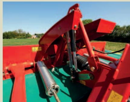
The headstock, design with the integrated Break-Away solution, helps the mower to clear obstacles.
