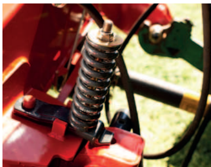
When encountering an obstacle the Non-Stop Break-Away system protects the cutterbar by swinging it back and up.
