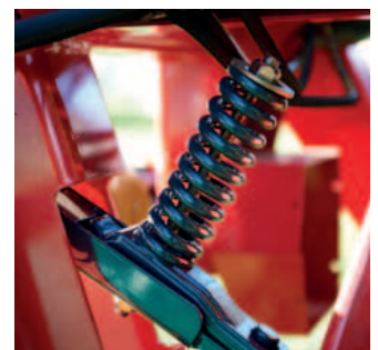
Break-Away device to protect the cutterbar against foreign obstacles.
