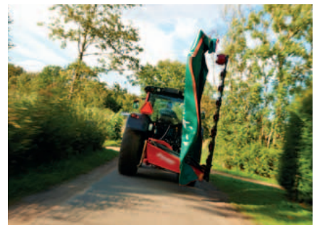
For transport the mower is positioned hydraulically into a vertical transport position.
