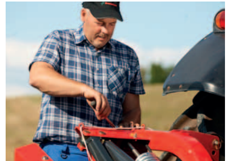
Ground pressure is easily set by adjusting the compensating spring.
