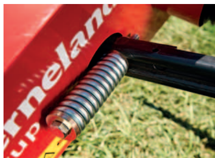
Break-Away device protecting the cutterbar when encountering obstacles.
