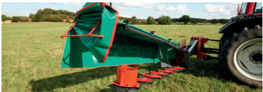
Easy access to the cutterbar for inspection and maintenance.
