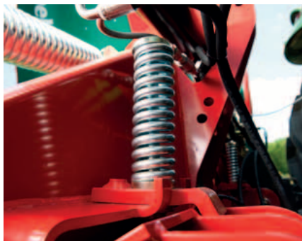
Non-Stop Break-Away system with auto reset.
