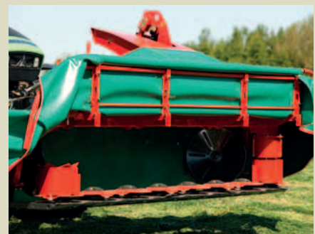
Easy access to the cutterbar with foldable front and side guards.
