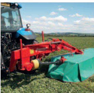
Hydraulic suspension for precise setting of ground pressure and superb adaptation.
