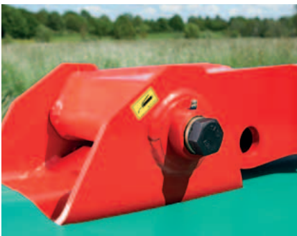
Two mounting positions of cutterbar on suspension for optimal overlap.
