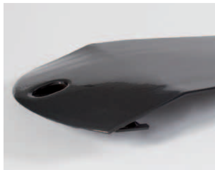
Smooth design of stone guards for improved cutting performance, particularly in laid and difficult crop.
