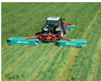
Centre suspended design for excellent ground following ability.
