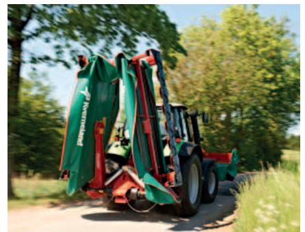
Vertical transport position for good weight distribution.
