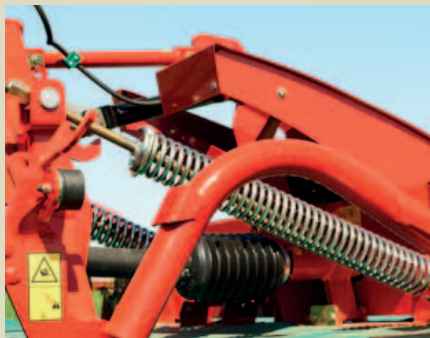
Two springs provide excellent ground following ability.
