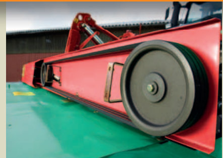
By switching pulleys changing between 1000 and 750 rpm is possible.
