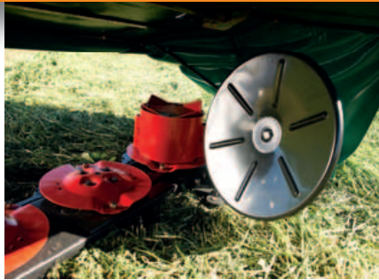
With the optional swath roller the swath is separated from the uncut crop.
