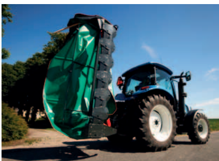
The 2300 series machines are folded hydraulically to a vertical position behind.
