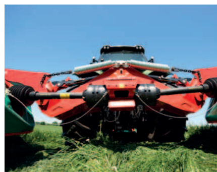
Two adjustable springs provide best possible ground adaptation.
