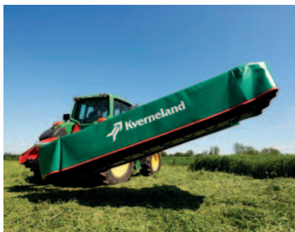
Lifting on headlands via hydraulic cylinder – ample ground clearance.
