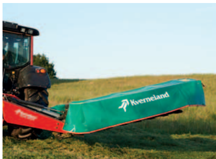
On headlands the mower is lifted without activating the 3-point linkage.
