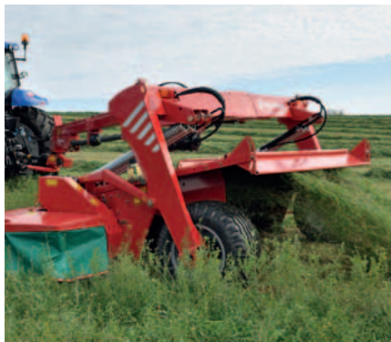
Operation on either left or right side – set from the tractor cab.
