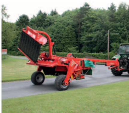
CT/CR models are swung to a central position behind the tractor for transport.
