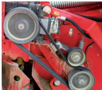
The conditioner is driven by 3 V-belts, providing smooth, silent power transmission to the rotor.
