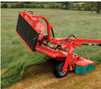
When placing the first swath, the BX-belt is raised and the hydraulically lowered for the second swath.
