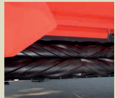
The rollers are manufactured from highly durable polyurethane, enabling both effective, uniform conditioning and long life span.
