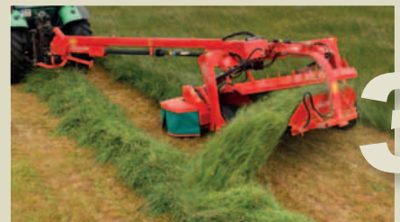
Two swaths into one with the Kverneland Taarup BX Auto-Swather for efficient pick up.
