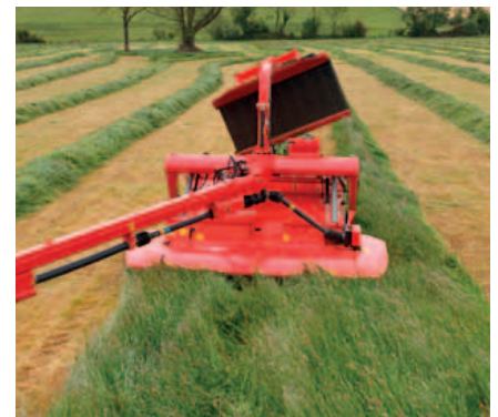
The belt is hydraulically suspended to reduce shock loads on the main frame and to give a more even swath formation.
