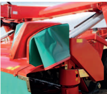
Easily foldable sideguards ensure narrow transport width.
