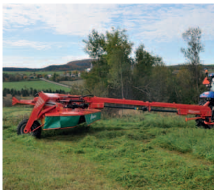
Centre pivot machines are easily manoeuvrable on headlands.
