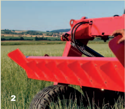
2 Changing from swathing to spreading is an easy operation. The rear plate is turned 180° (no tools required).
