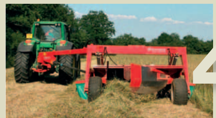
Two narrow swaths placed alongside each other with the swath deflector.
