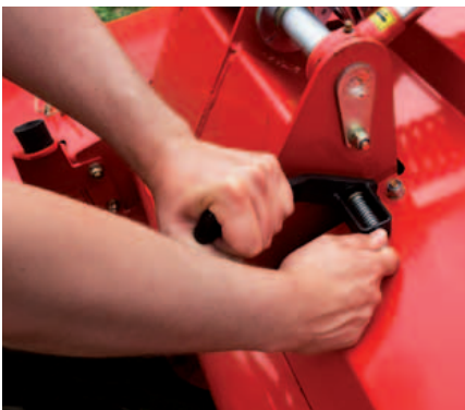
The conditioner plate can be set in 3 positions according to the required conditioner effect.
