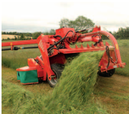
During the second pass, crop can be placed on top of the first one, or as shown here side by side.
