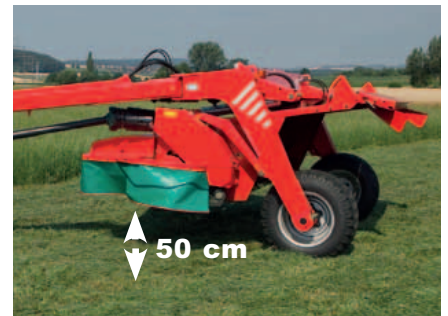
Clearance of 50 cm due to the design of the trolley.
