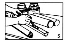
5) Grease the male joint section and reassemble protection
