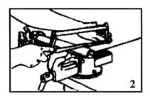
2) Cut the excess length of both tubes
