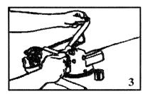
3) Deburr and clean the saw-dust off ends of tubes. Remove packing inside shaft tubing
