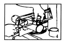
4) Cut the plastic protection to the same length you have cut the joints
