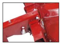
Wheel axles are attached by heavy duty pivot pins with replaceable bushings that extend through the cutter strongbacks. This dependable mounting arrangement provides extra strength and less pivot pin wear.
