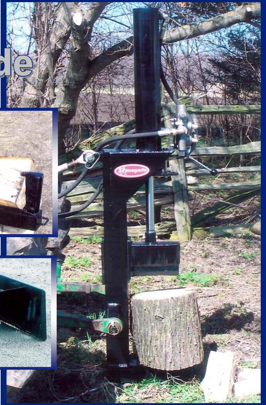
3ph Vertical 20 Ton Push, 4 x 24 Cylinder
