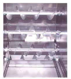
This same "farmer-driven" change is happening with the stainless steel auger flighting. Introduced in 1988, the stainless auger is now firmly in place as the preferred auger; all carts built have at least some stainless augers, and the "topof-the-line" carts have all augers made with stainless steel flighting.
