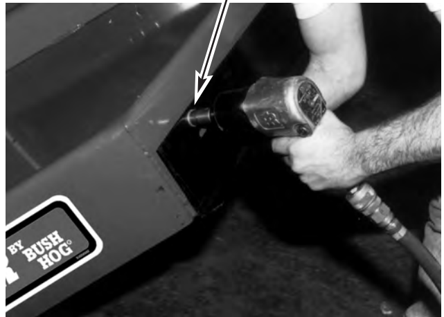
Figure 5-9 Rear Band Installed
