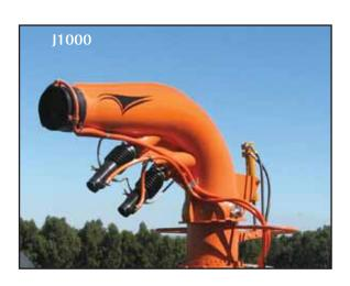
• The main duct on the J -1000 can be adjustade both horizontally and vertically. It also has two auxiliary ducts to cover the area close to the tractor, thus improving the quality of spray applications.
