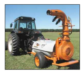
Different working conditions lead us to adopt the following criterion for choosing the tractor that will drive the J-1000 cannon sprayer.
