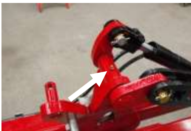
Ground follower adjustment right axle
