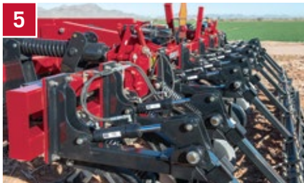
5 Crumbler pressure: achieve consistent clod sizing
