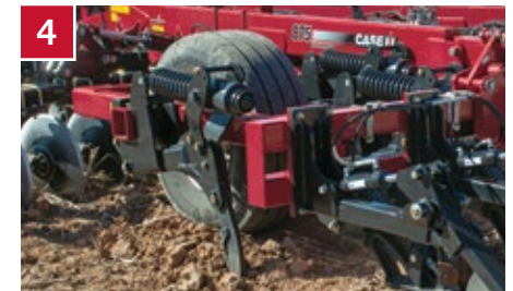
Shank depth: target the compaction layer
