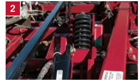
Disk gang pressure: reduce pressure on frame
