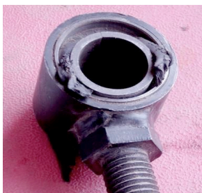
Old/Worn Bushing System
