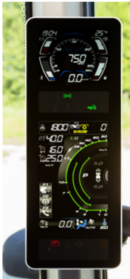
THE NEW MF VDISPLAY. The MF 8S's easy to read digital dashboard can be personalised.
