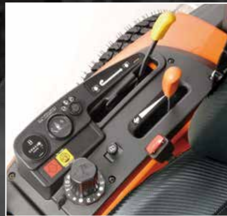
1/4" Increment Cutting Height Adjustment
