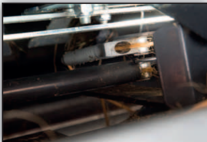
Twin tube fast operating twine binding system.
