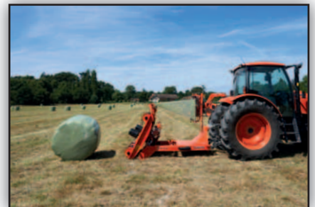
Drop the wrapped bale - all controlled via the optional remote control.
