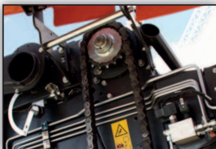
The main bale chamber drive is a heavy duty pitch chain. This allows for a longer lifespan and reduced maintenance.
