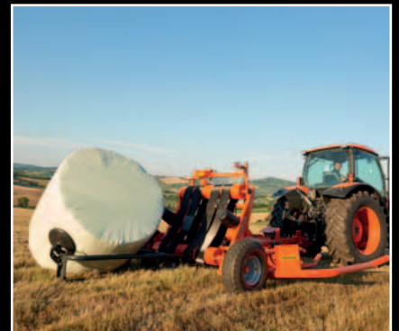
The Kubota WR1400 can be fitted with a bale on end kit. The bale is tipped off gently without damaging the bale.
