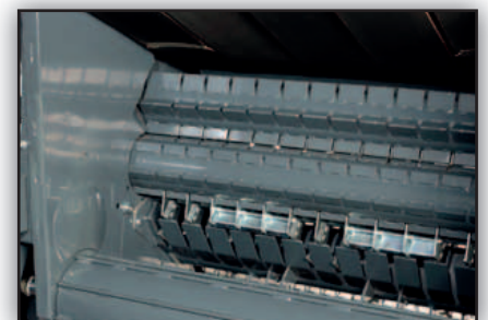
The two front rollers with self-cleaning scrapers are designed to work well in silage and provide instant bale formation. The scrapers efficiency keeps the rollers free from wet silage building up.
