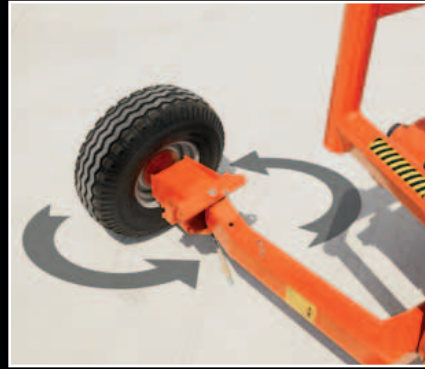
For narrow transport width, the right hand wheel is turned to the inside of the support arm.
