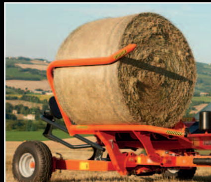
Hydraulically operated loading arm with a low loading height provides fast transfer of bale from arm to turntable.
