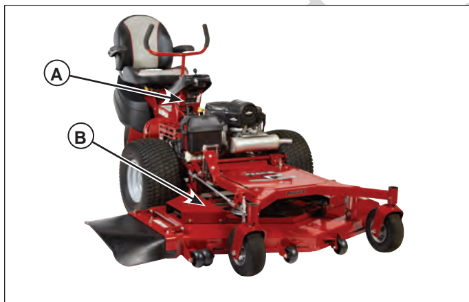
Figure. 1 Location of Identification Tags. A. Powerhead Identification Tag B. Mower Deck Identification Tag
