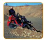
boom lift and bucket dump functions are controlled by a single joystick.
