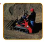
comes equipped with two separate boom mounted hydraulic circuits. One circuit operates cylinder equipped attachments such as grapples and 4:1 buckets. The second hydraulic circuit equipped with integrated motor spool is used to power and protect motor driven attachments such as sweepers and snow blowers.
